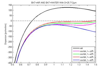
**Fig.5** Dispersion characteristics with different temperature of water with total diameter of 25.712μm.
