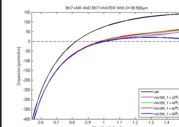
**Fig.6** Dispersion characteristics with different temperature of water with total diameter of 38.568μm.
