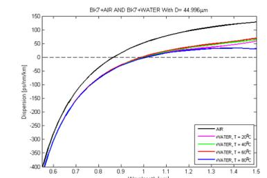
**Fig.7** Dispersion characteristics with different temperature of water with total diameter of 44.996μm.
