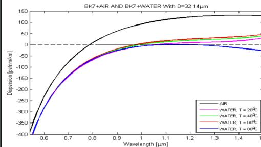
**Fig.2** Dispersion characteristics with different temperature of water with total diameter of 32.14μm.
