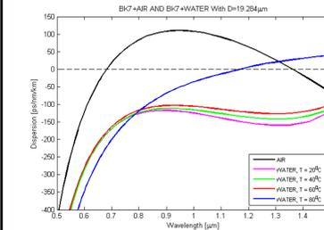
**Fig.4** Dispersion characteristics with different temperature of water with total diameter of 19.284μm.
