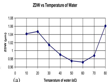
**Fig.3** Dependence of ZDW (a) and ZDWS (b) on temperature of water.
